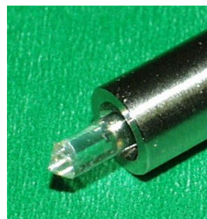
Figure 3: Close-up of the zinc sulfide ATR head
