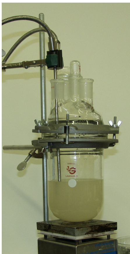
Figure 1: Fermentation reactor with ReactionView probe
